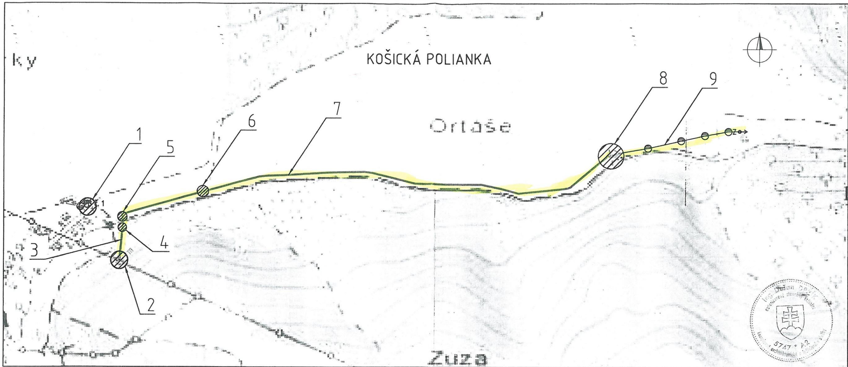
1. ÚPRAVA DOMOVEJ PRÍPOJKY PRE RD p. č. 427/6 - PODZEMNÝ KÁBEL AYKY-J 4x16+2,5 (l=25M) - MONTÁŽ
